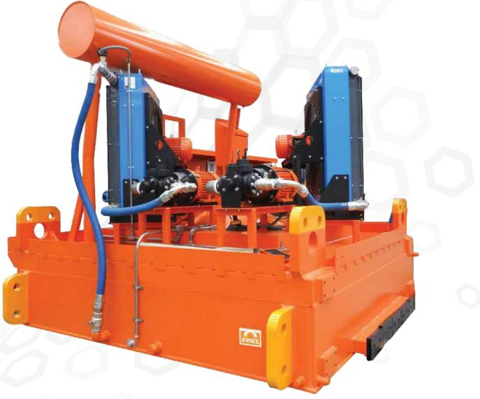
Successfully removes damaging tramp from flows of coal, limestone, sand, gravel, municipal waste, wood products, recycled materials, other ores and almost any conveyed non-ferrous material
