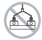
No hooking of two lifting magnets without the use of a properly designed spreader beam.
