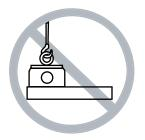
Care should be taken to make certain the load is correctly distributed for the lifting magnet being used.
