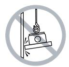
Do not allow load or magnet to come into contact with any obstruction.
