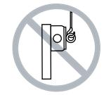
Avoid placing the magnet in shear.
