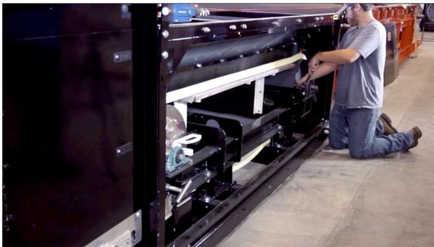
The videos feature [RevX-E Eccentric Eddy Current Separators](#), which are designed with an eccentrically mounted magnetic rotor within a non-conductive shell to separate nonferrous metals. The rare earth rotor produces a powerful and focused field at the end of the belt.
