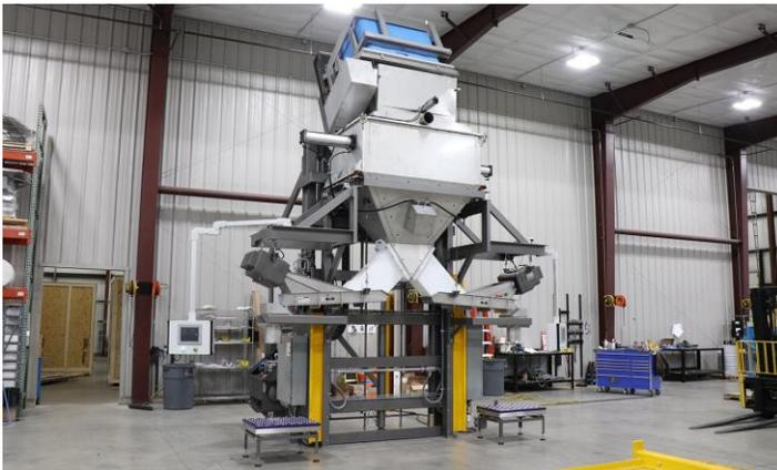
As a global pandemic raged, [Material Transfer](#) was called upon to engineer a solution to maintain ice pellet size consistency, meter ice evenly to protect each vaccine, and monitor ice discharged during packaging, all while automating the process. The integrated process includes a crusher, scale system, and customized feeder and controls required to report diagnostics to the vaccine manufacturer.
