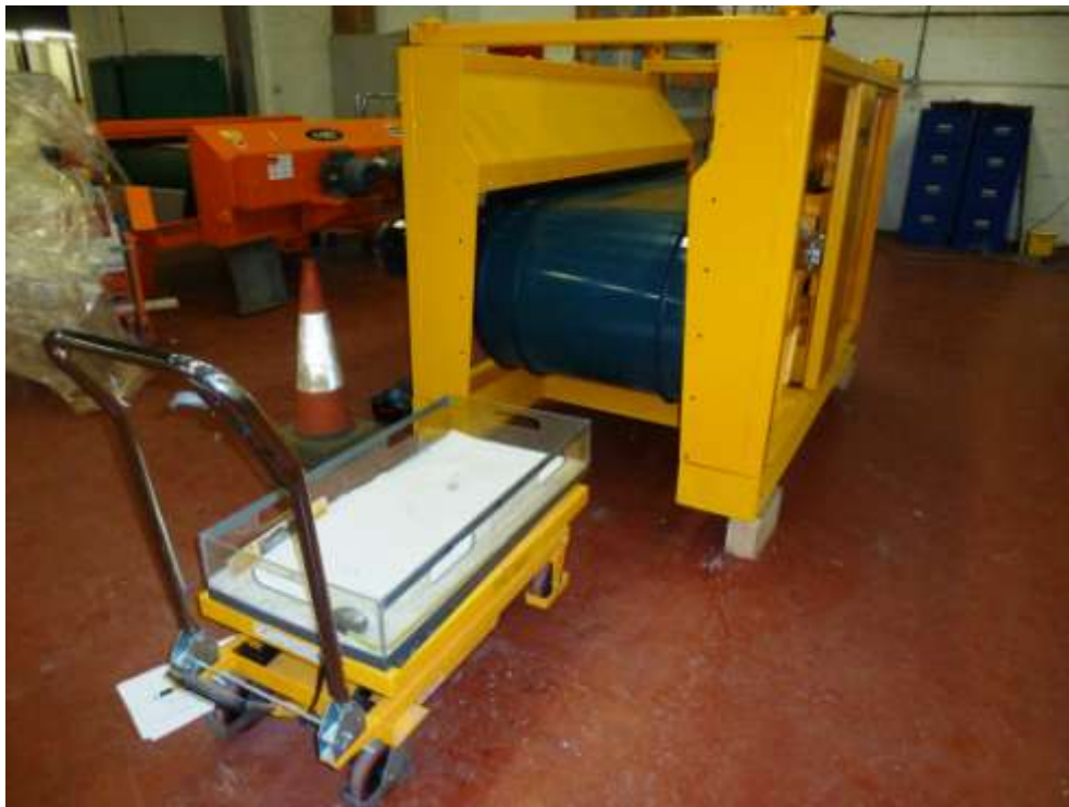
Figure 18 Catch-Tray in Position in front of Steinert ECS
