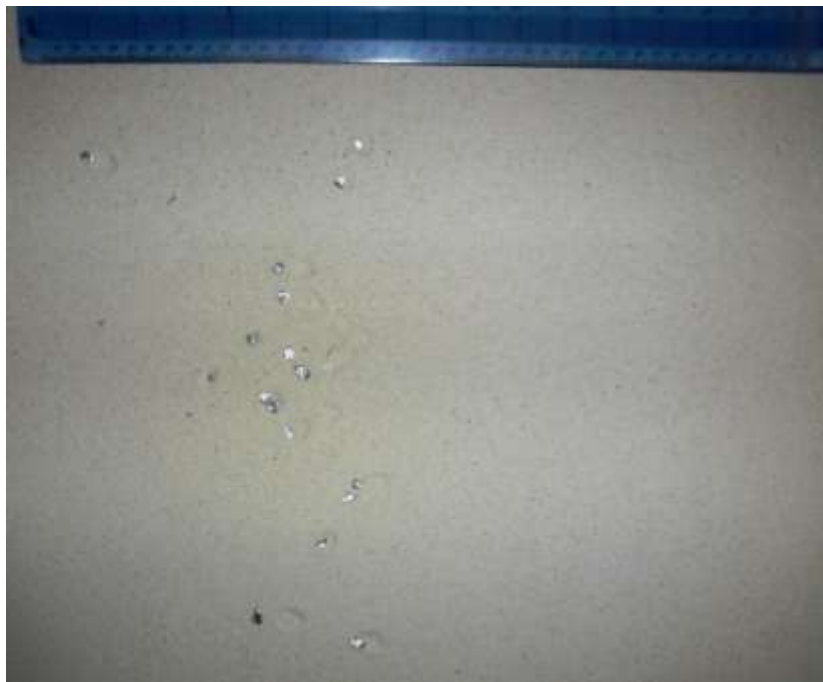
Figure 16 Flat Aluminium Particles in the Catch-Tray Showing Initial Impact Sites
