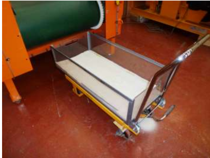
Figure 9 Perspex Catch-Tray Filled with Glass Sand to Catch the Test Pieces Deflected by the ECS
