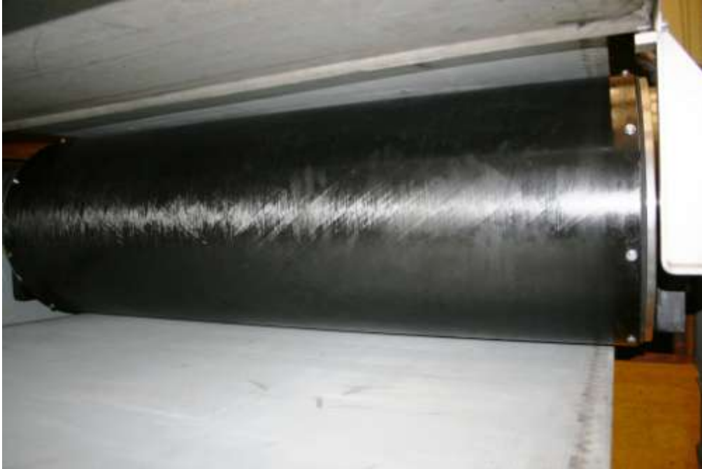
Figure 5 Eriez ST-22-C Fitted with a High Technology Material Shell
