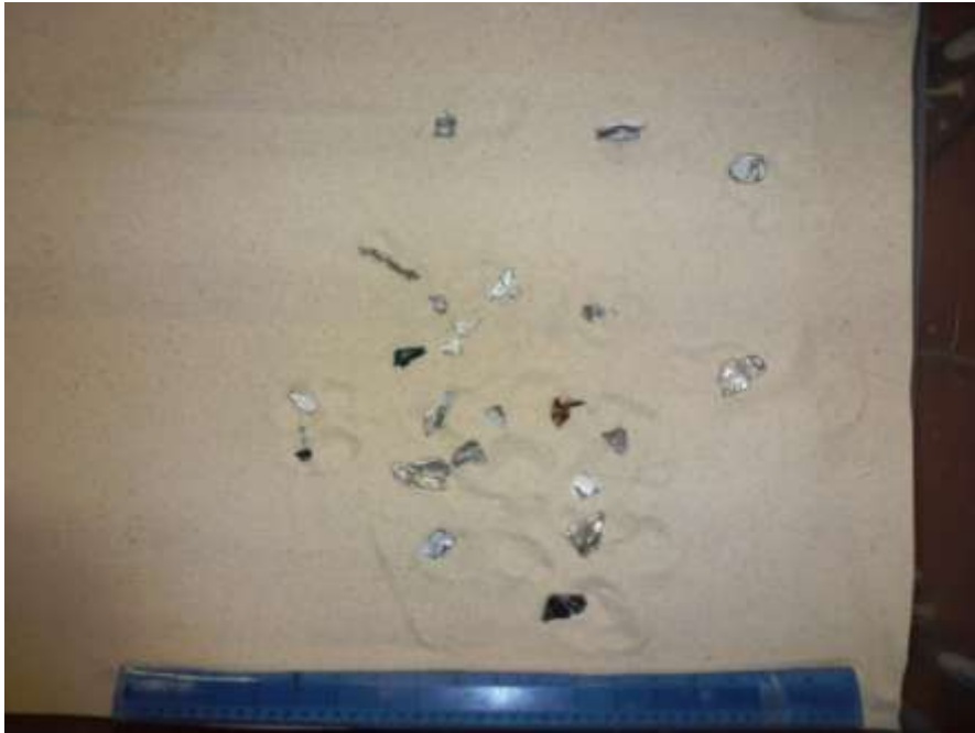
Figure 15 Typical Disposition of Small Fragmentised Aluminium after Test
