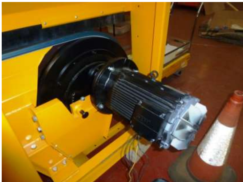
Figure 8 Detail of Steinert Eccentric Rotor Adjustment Mechanism in the 22° Position
