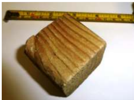
Figure 12 Large Piece of Wood used as a Non-Metallic Test Piece
